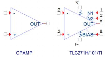
b. In addition to the feedback resistors needed for your inverting amplifier, you must explicitly connect the ±5 V DC power supplies to the op-amp, like this:
