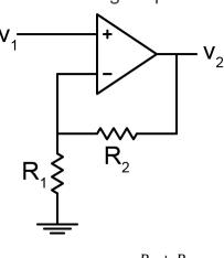
$$v_2 = \frac{R_1 + R_2}{R_1} v_1$$
