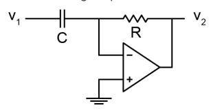
$$v_2 = -RC\frac{d}{dt}v_1\hat{V}_2 = -j\omega RC\hat{V}_1$$
